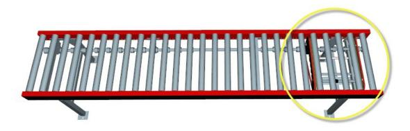
Make sure to divide the different parts that has to be handled separately. In this example the component contains a roller conveyor and a transfer belt – we are going to control the transfer belt by a pneumatic device (lifting up and down).
